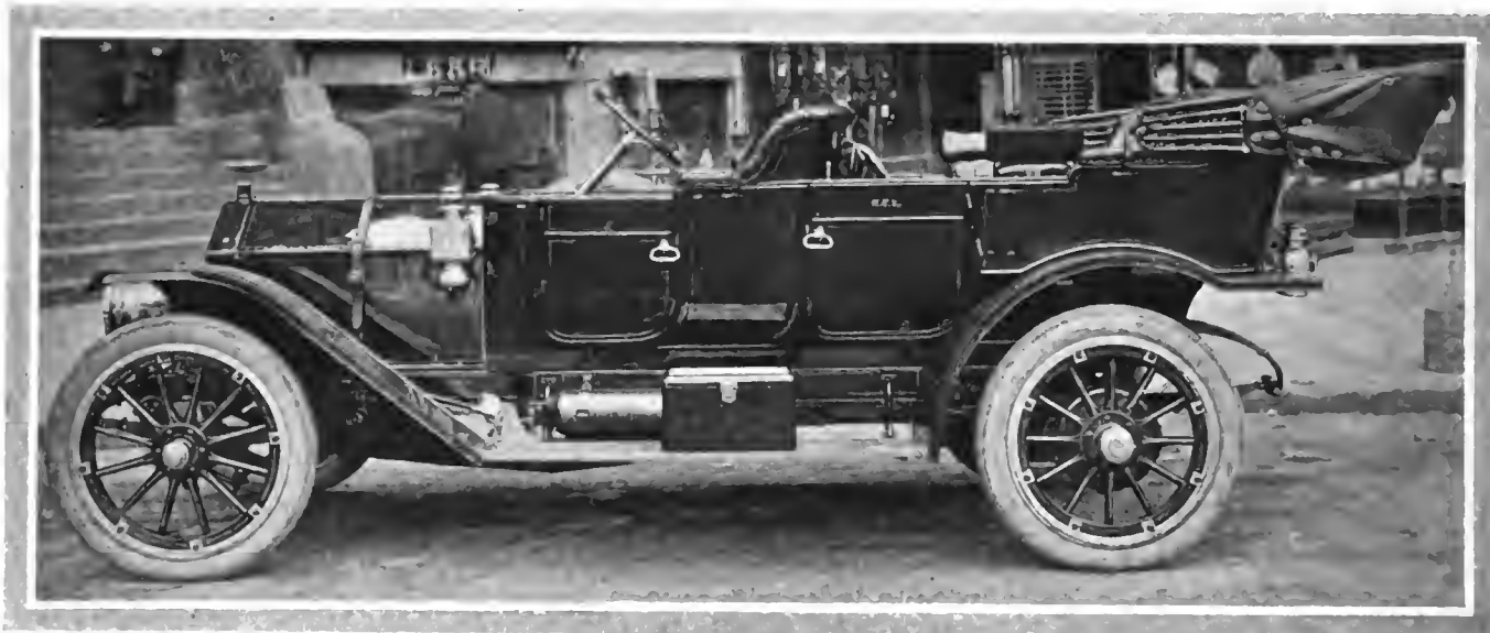
Model M 1911. Fore-door type of touring car, seating seven passengers, showing a well-fitted top folded down, and other advanced features
